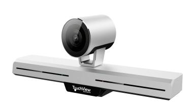
The TouchView Enterprise PTZ Camera features a wide angle no distortion lens, ultra-high definition, 360 degree rotated EPTZ, a folding bracket, and USB 3.0 connection.
